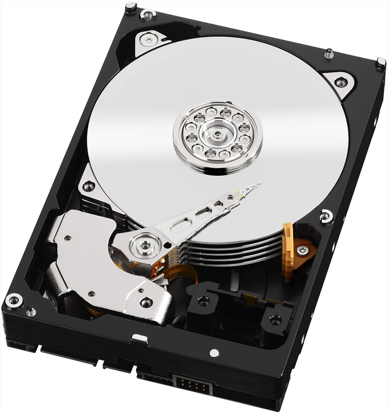
Figure 2.4: An open view of a hard disk drive, showing the platters, read/write heads, and internal components.
