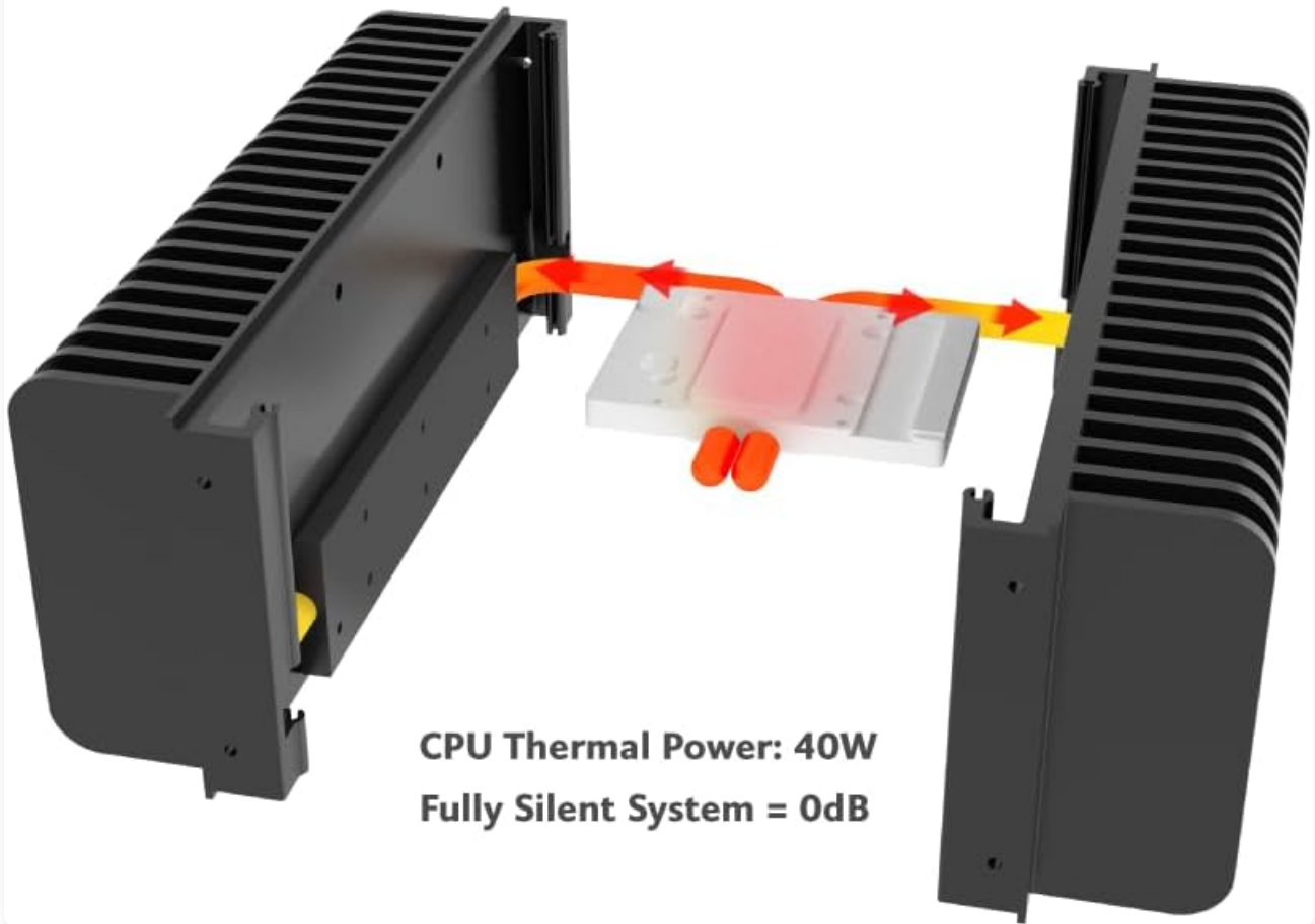
Figure 3: Diagram illustrating the internal passive thermal module with 8mm copper heat pipes, designed to transfer heat from the CPU to the case's fins for silent cooling up to 40W TDP.
