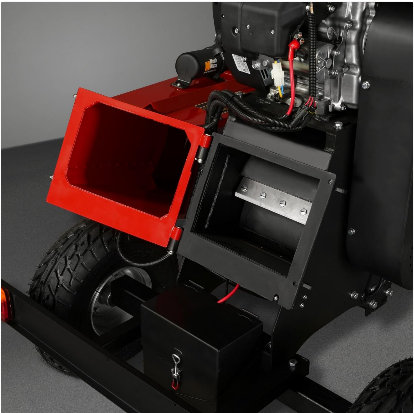
Figure 5.1: View of the chipping mechanism, showing blades and anvil.
