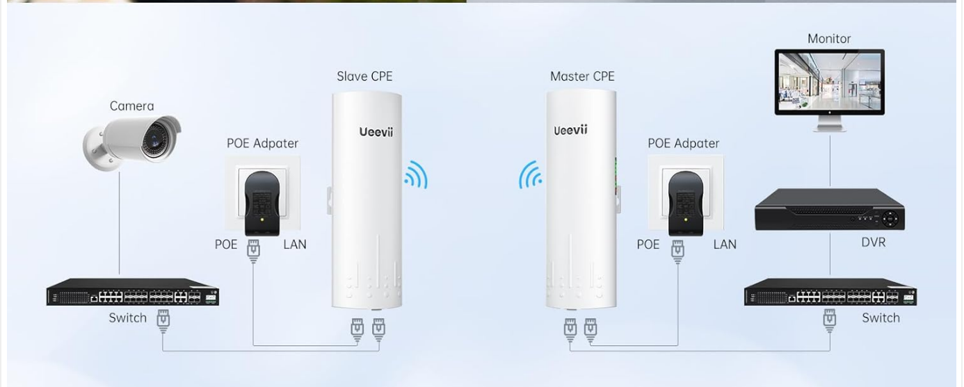
Figure 3.2: Example setup for extending a monitoring system using CPE450 bridges.
