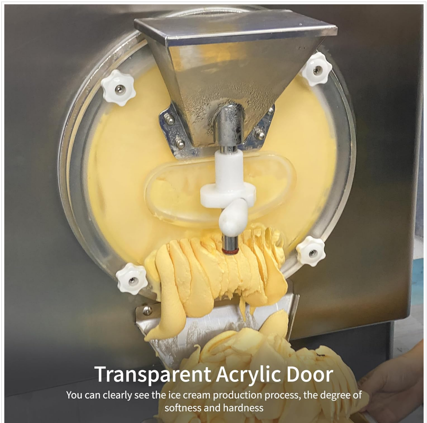
Figure 6: The transparent acrylic door allows for clear visibility of the ice cream production process, enabling monitoring of consistency.
