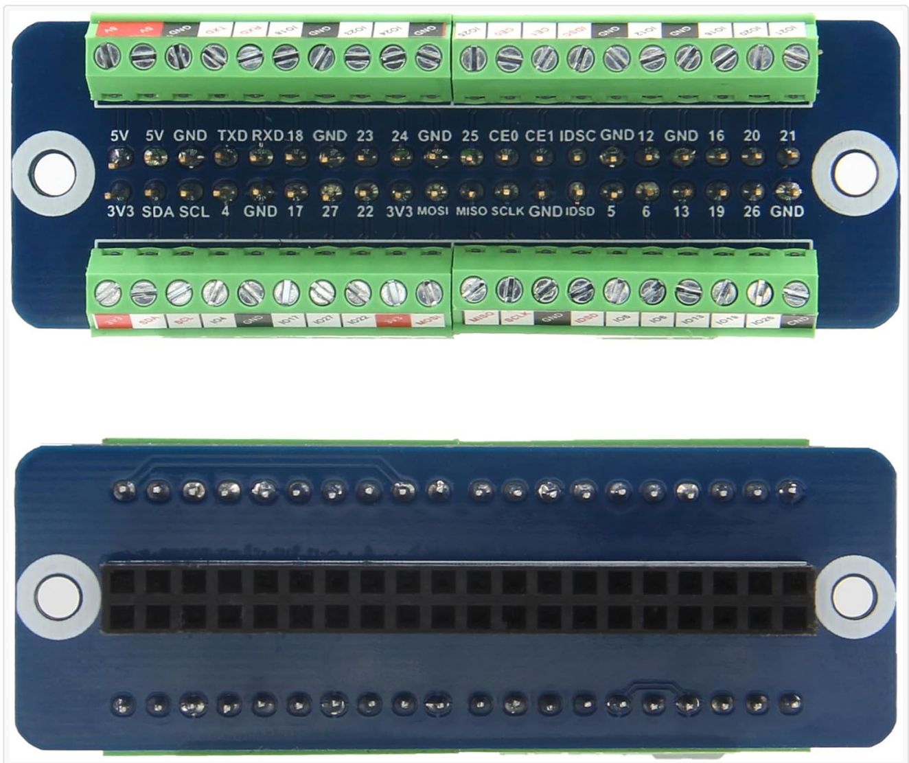
Image: The Geekworm G469 GPIO Terminal Block Breakout Board, as included in the package.
