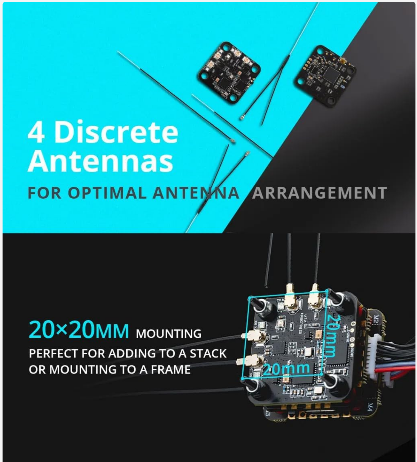
Figure 6: Visual representation of the DBR4's 20x20mm mounting holes and the recommended arrangement for its four discrete antennas to achieve optimal signal reception.
