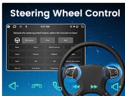
Figure 5.9: The car stereo's interface for learning and configuring steering wheel controls, showing various assignable functions.
