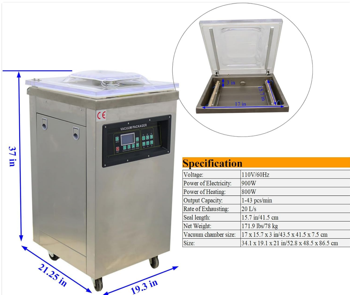
Figure 3.1: Machine dimensions and key specifications. This image provides a visual representation of the machine's overall dimensions and lists important technical parameters.
