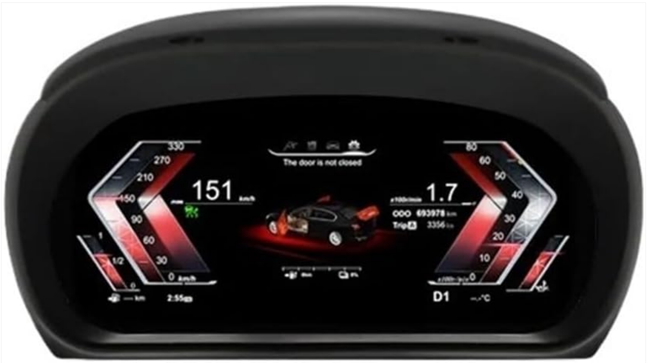
Figure 2.1: The TKNSHYDW 11-inch LCD Digital Instrument Cluster in operation, displaying key vehicle data such as speed, RPM, and a visual representation of the car's status, including an open door warning.
