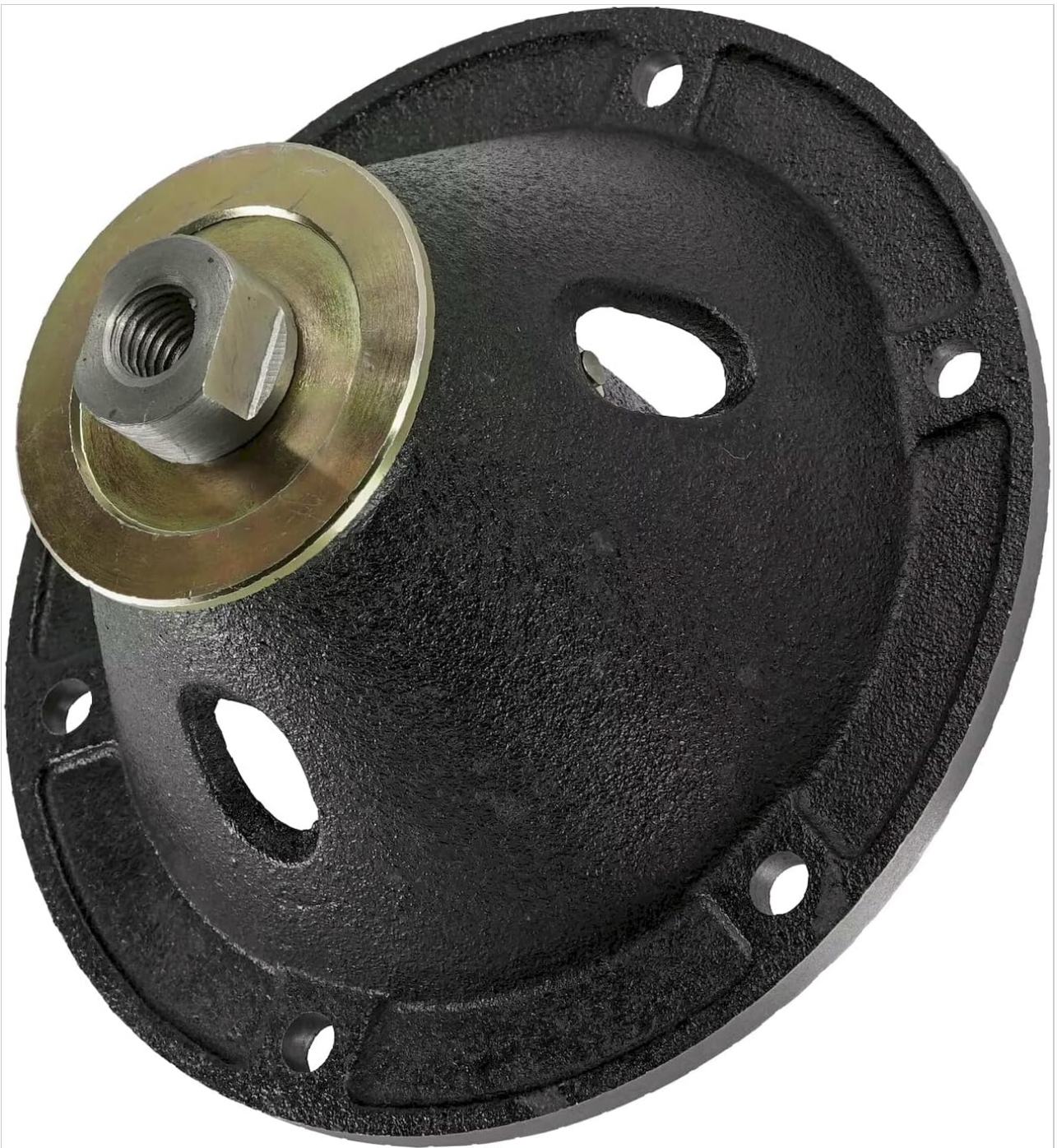
Image 1: Top-down view of the cast iron blade deck spindle. This image highlights the robust cast iron housing, the central shaft with its securing nut and washer, and the four precisely drilled mounting holes on the flange, essential for secure attachment to the mower deck.
