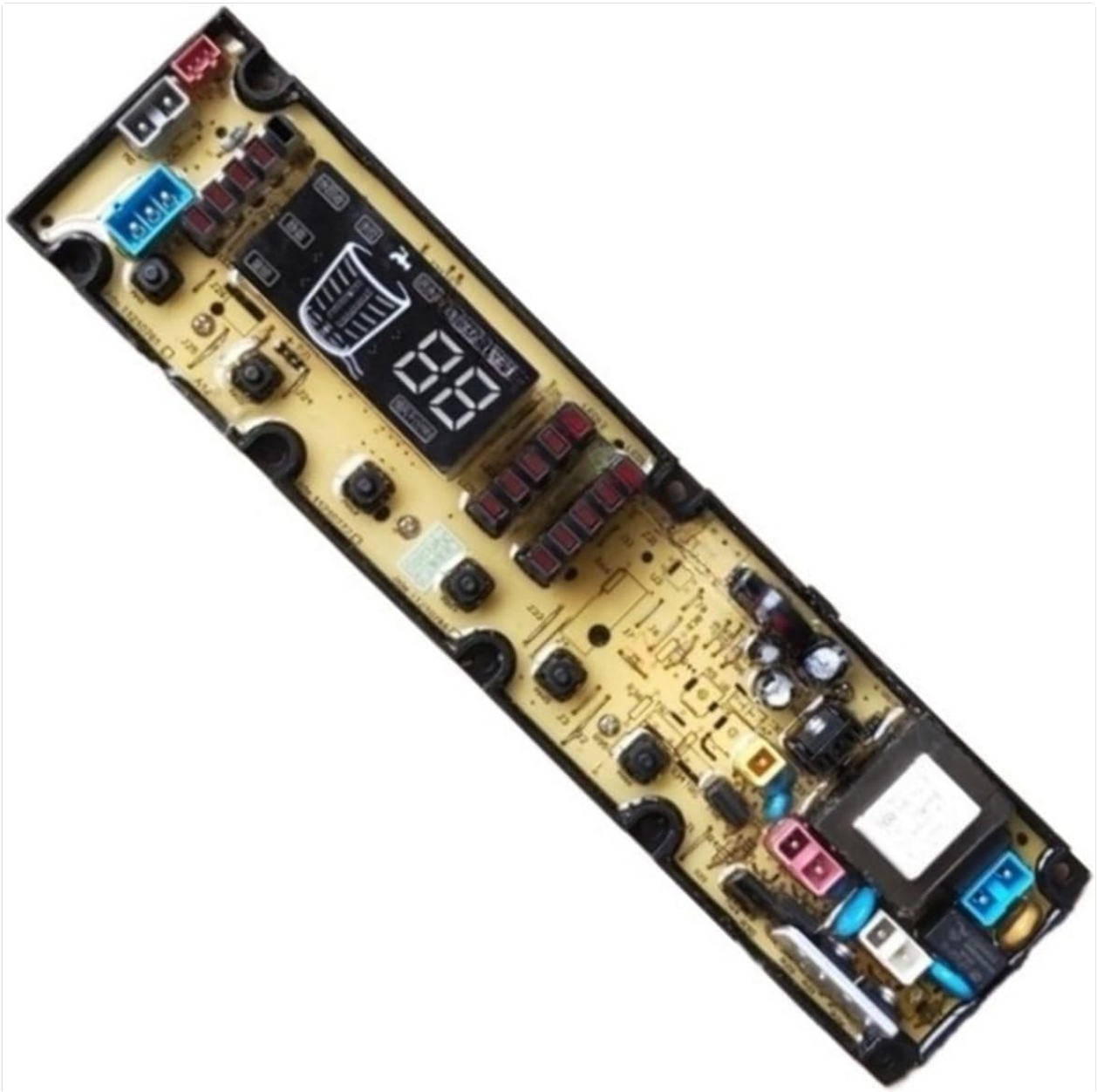
Image 1: Angled view of the WEIFUS Daewoo Washing Machine Control Board DWF-A1088 / 11210761, showing various connectors and electronic components.
