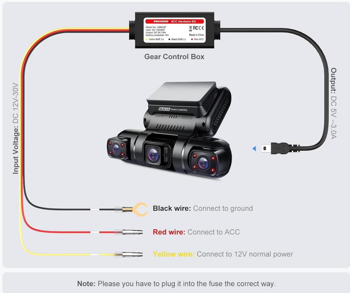
Image 4.1: Wiring diagram for the ACC Hardwire Kit connection to the vehicle's fuse box.
