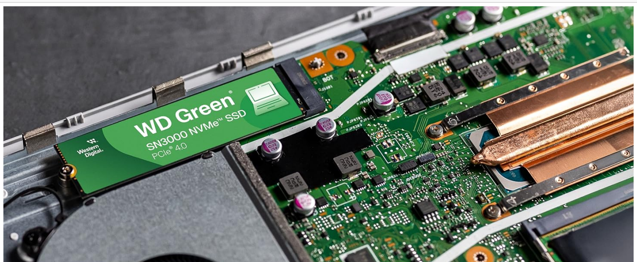
Image: The WD Green SN3000 NVMe SSD installed in an M.2 slot within a laptop, showing its green label and secure fit.
