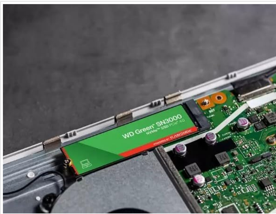
Image: The WD Green SN3000 NVMe SSD installed in an M.2 slot within a laptop, showing its green label and secure fit.
