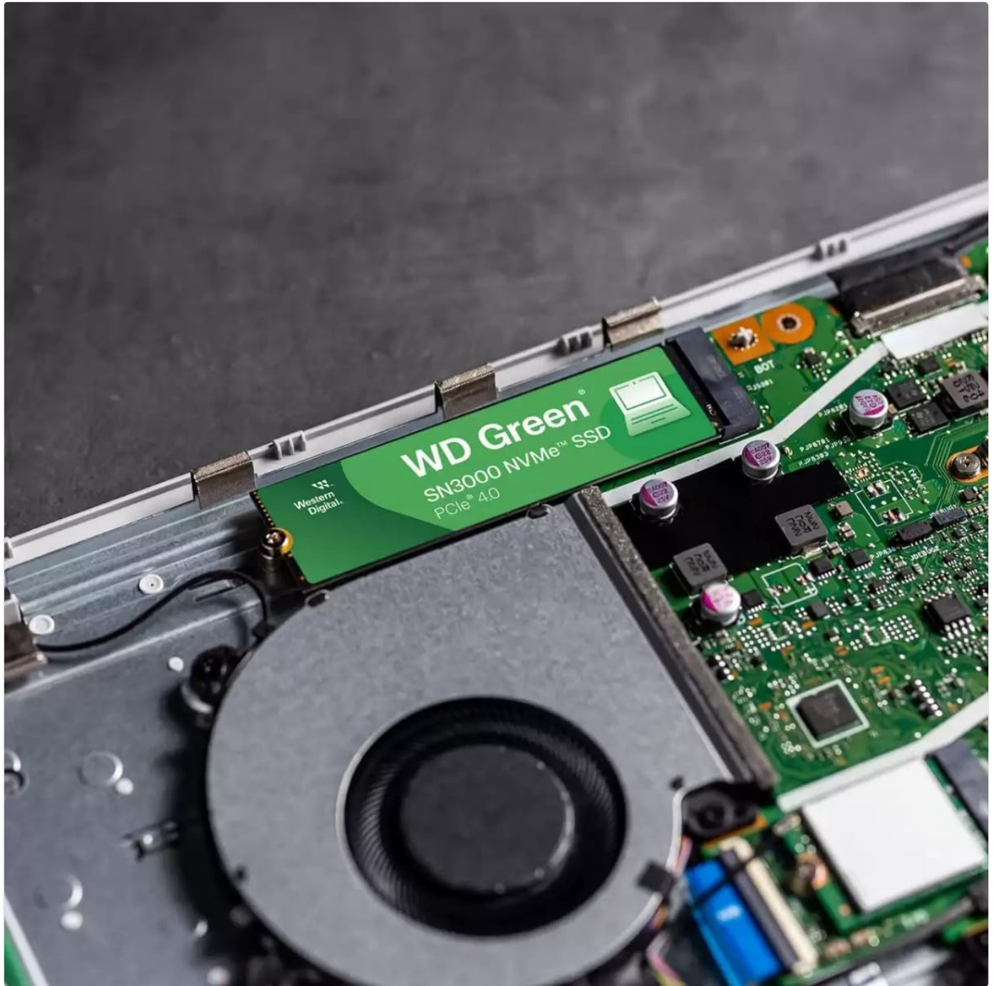
Image: The WD Green SN3000 NVMe SSD securely installed in an M.2 slot on a laptop's motherboard, surrounded by other internal components.
