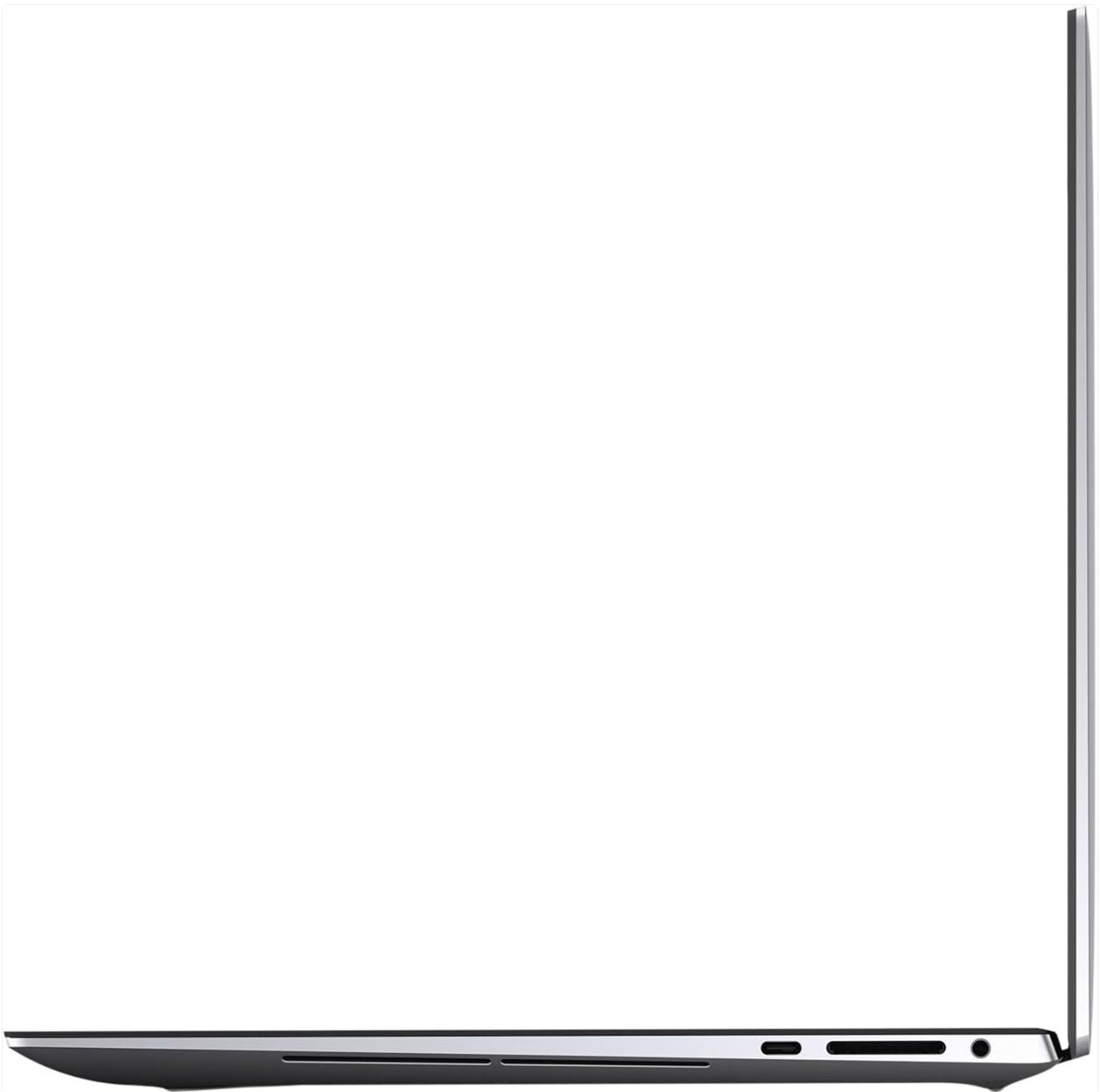
Figure 3.2.2: Right side of the Dell Precision 5560, featuring a USB 3.2 Gen 2 Type-C port with DisplayPort Alt Mode, a Secure Digital card slot, and a headphone jack.
