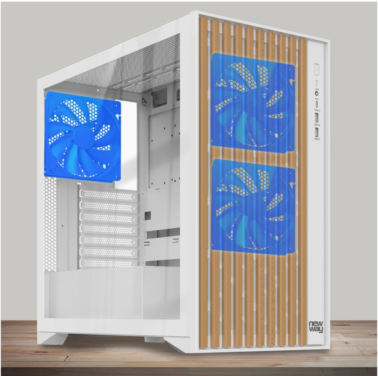
Image 3.4: Diagram indicating potential fan mounting locations, including the pre-installed front fans and a rear exhaust fan.
