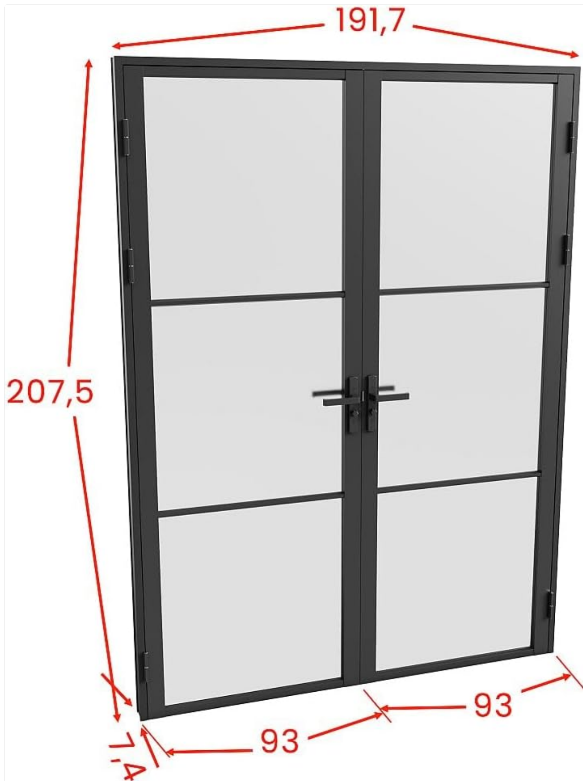
Image 4.1: Dimensional diagram of the MASERU door block, indicating height, width, and depth.
