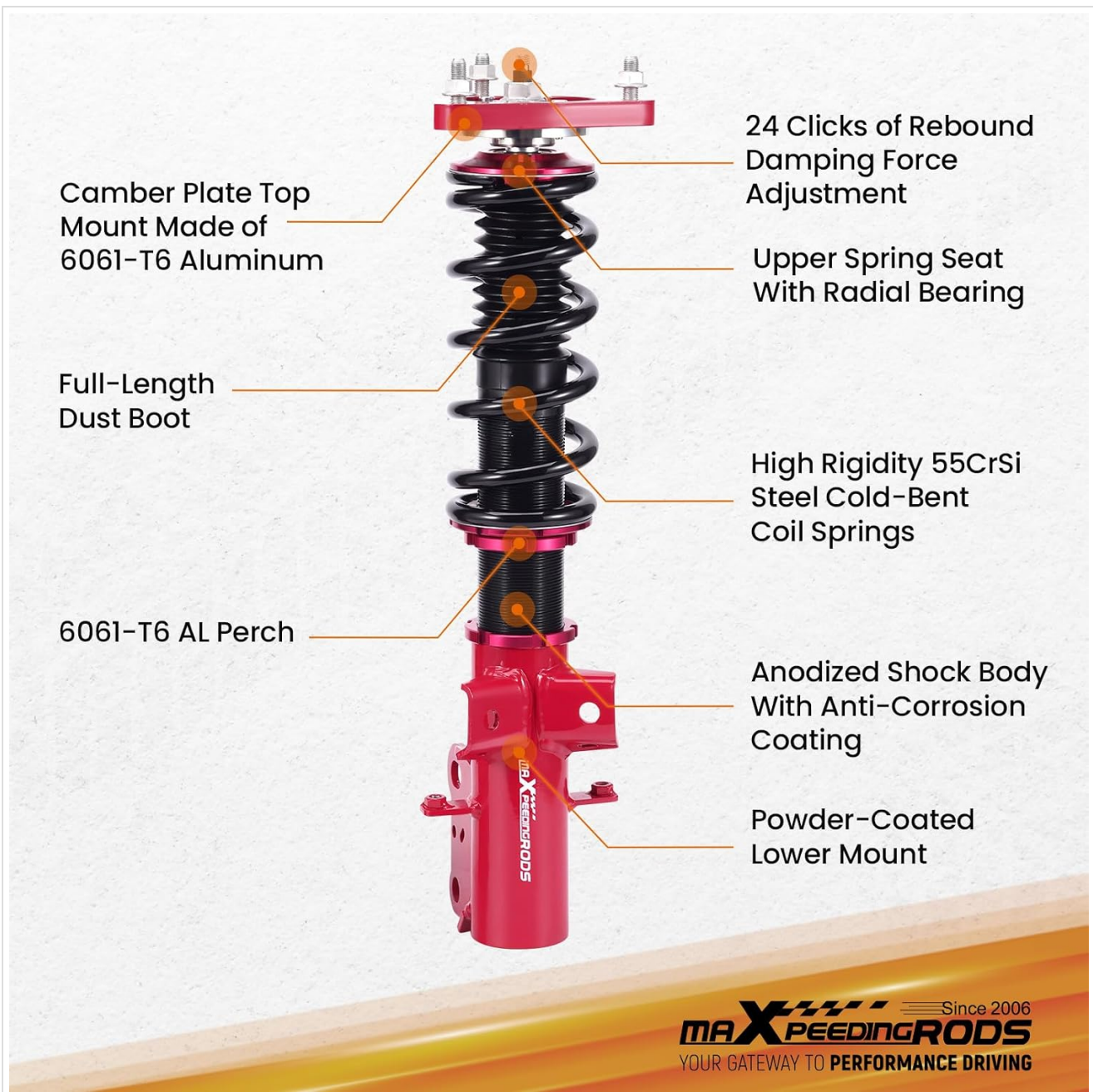
Image: A detailed diagram of a coilover unit, highlighting features such as the camber plate top mount (6061-T6 Aluminum), 24 clicks of rebound damping force adjustment, upper spring seat with radial bearing, full-length dust boot, high rigidity 55CrSi steel cold-bent coil springs, 6061-T6 AL perch, anodized shock body with anti-corrosion coating, and powder-coated lower mount.
