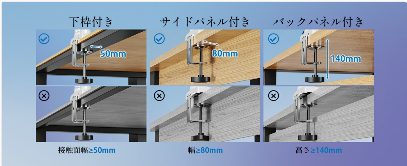
Clamp installation details for various desk configurations.
