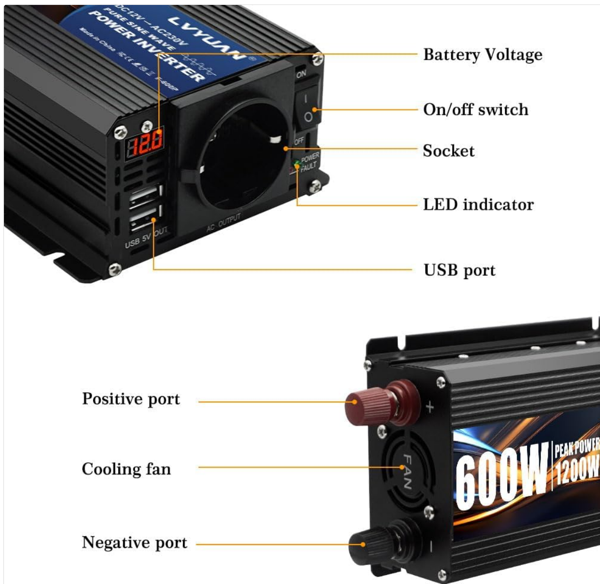
Image: This diagram highlights the key components of the inverter, including the battery voltage display, on/off switch, AC output socket, LED indicator, USB ports, positive and negative DC input terminals, and the cooling fan.
