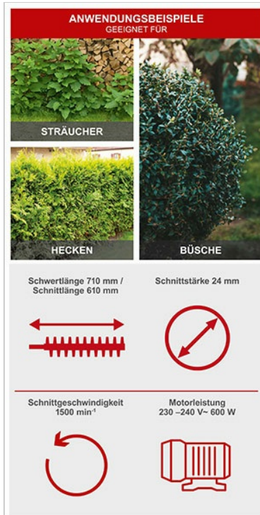
Figure 8.1: An overview of the key technical specifications, including blade length (710mm), cutting length (610mm), cutting thickness (24mm), cutting speed (1500 min -1 ), and motor power (600W).
