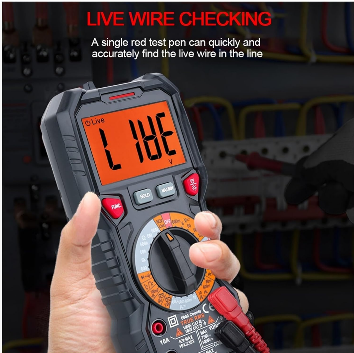
Figure 4: Live wire checking function in use. The display indicates "LIVE" when a live wire is detected, accompanied by an alarm.
