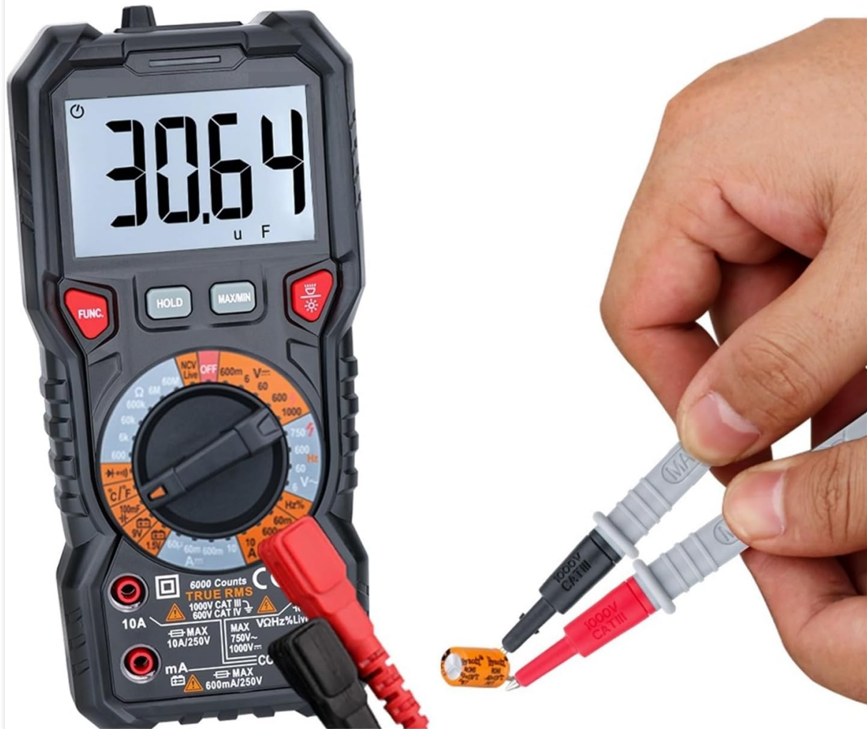
Figure 3: Performing a capacitance test. The display shows a reading in microfarads (uF).
