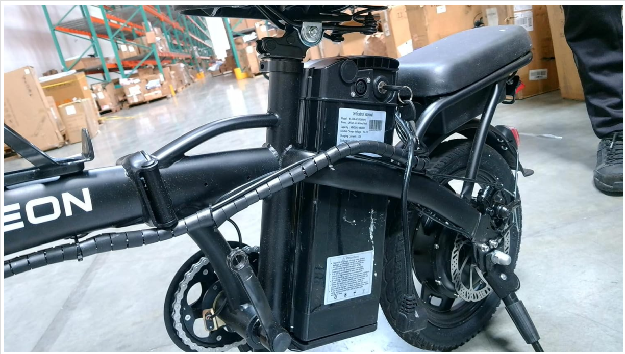
Figure 4.3: Close-up view of the removable battery compartment on the DEEPOWER electric bike.
