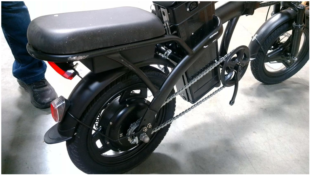
Figure 6.1: View of the rear wheel, motor, and chain, areas requiring regular inspection and maintenance.
