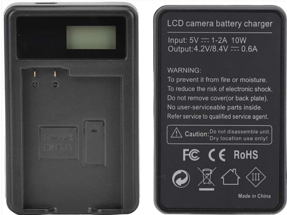
Image 2.1: Charger with warning labels
