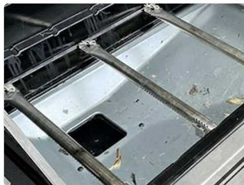
Image: Burners correctly installed.
