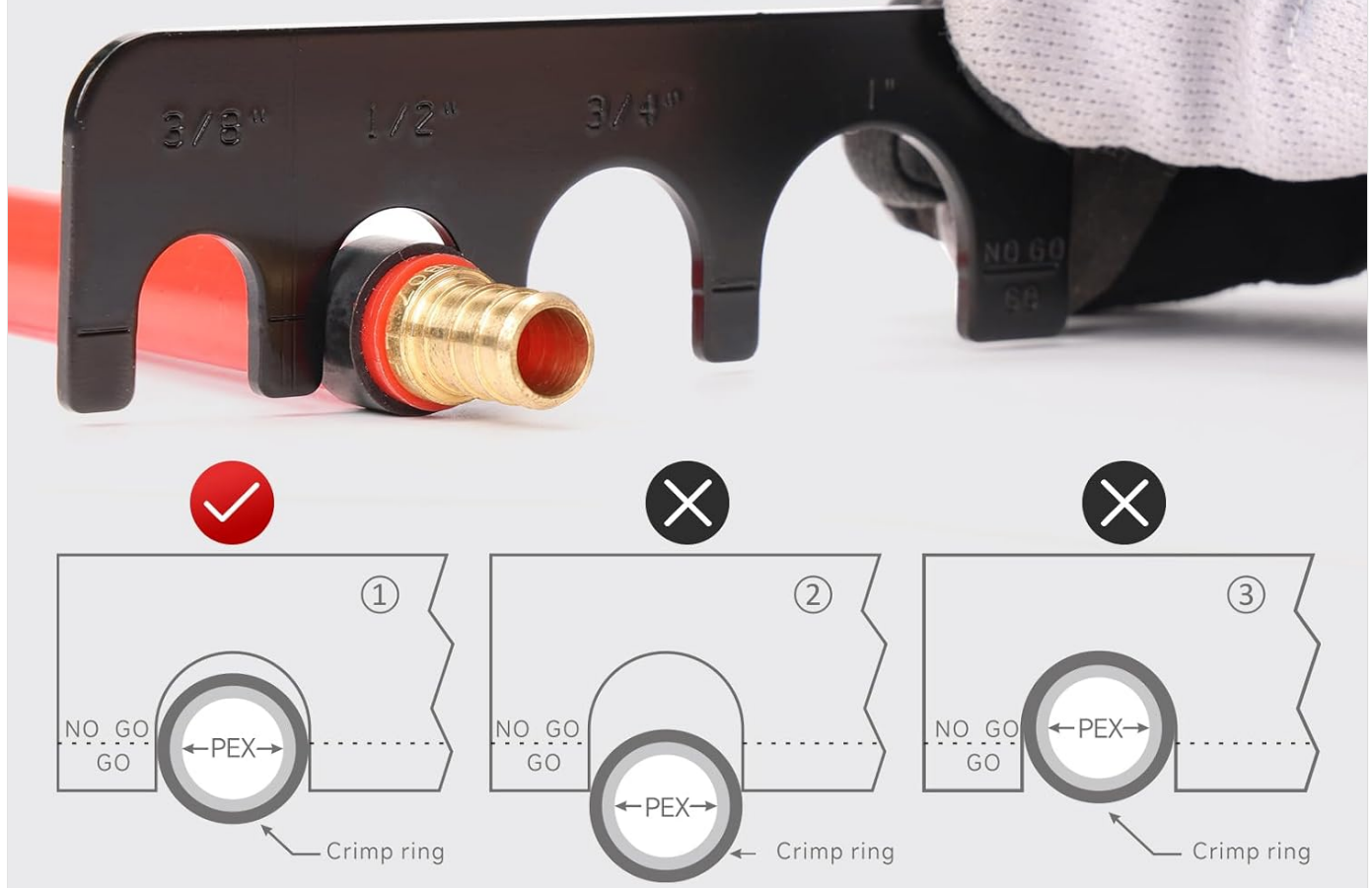
Figure 4.3: Proper use of the Go/No Go gauge for crimp verification.
