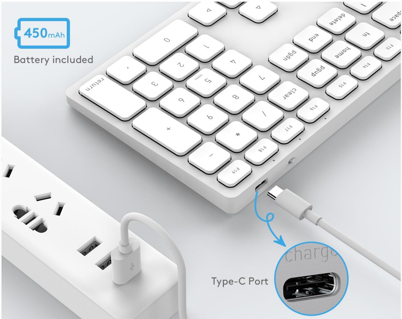
Image 3.1: The keyboard connected to a power source via its USB-C charging port.
