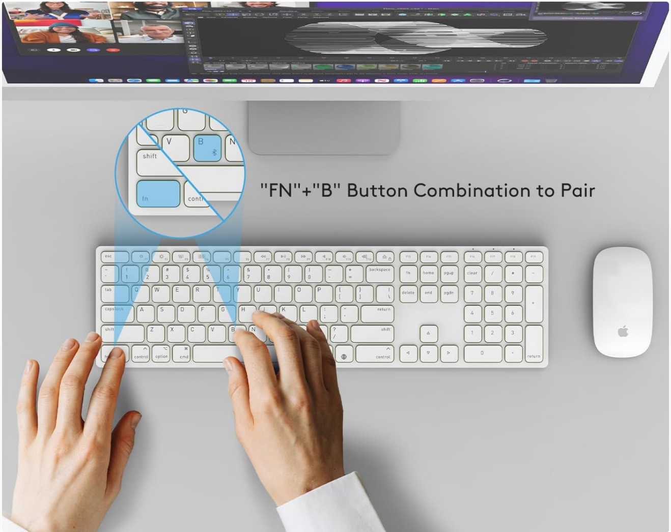
Image 3.3: Illustration showing the "Fn" + "B" key combination for initiating Bluetooth pairing.
