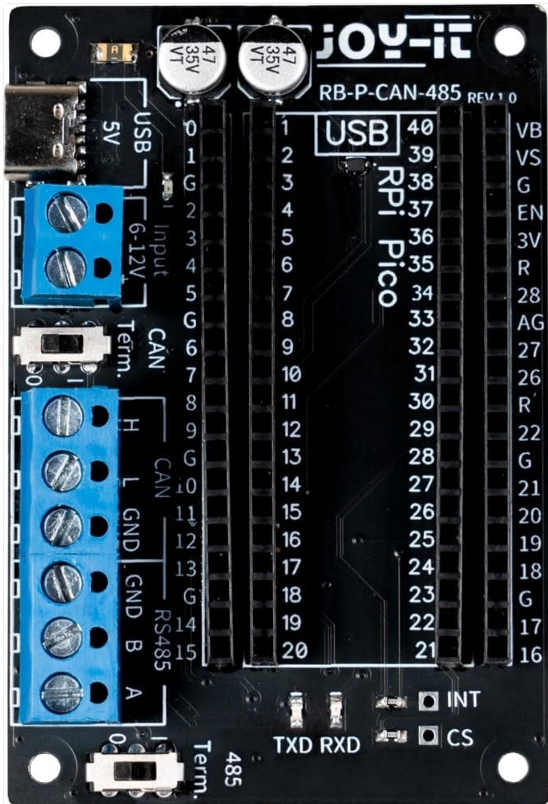
Figure 2: Top-down view of the Joy-it RB-P-CAN-485 Module. This image clearly labels the USB-C port and the screw terminal for power input, as well as the CAN and RS485 connections and the Raspberry Pi Pico pinout.
