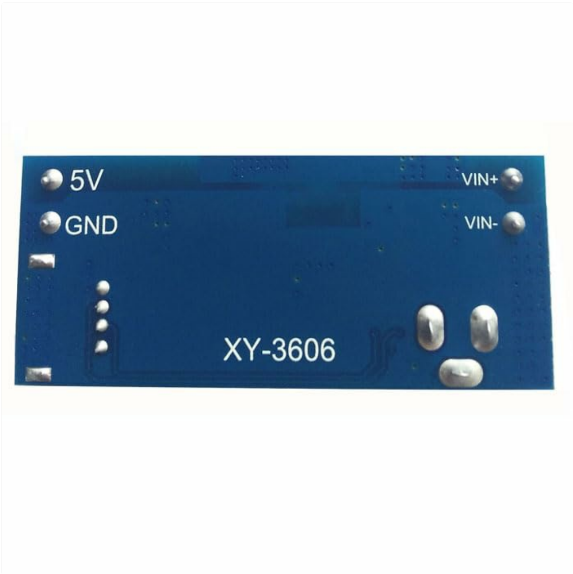
Figure 3.4: Bottom view of the buck converter module, displaying the model identifier XY-3606.
