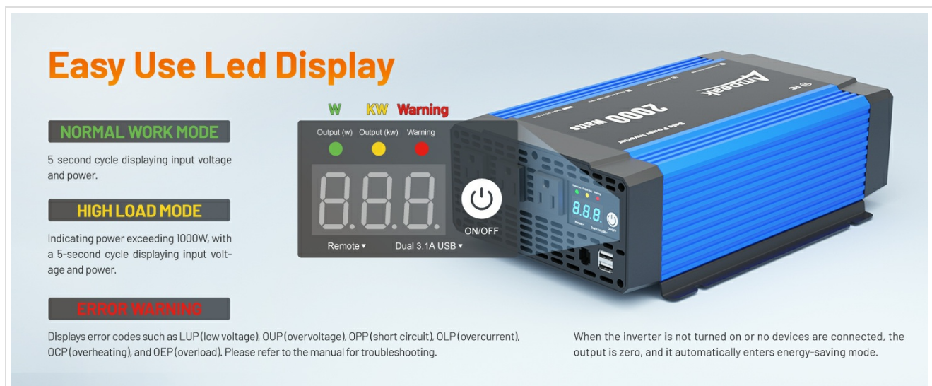
Figure: The LED display on the Ampeak 2000W Inverter, illustrating how it shows normal working status, high load mode, and error warnings for easy monitoring.
