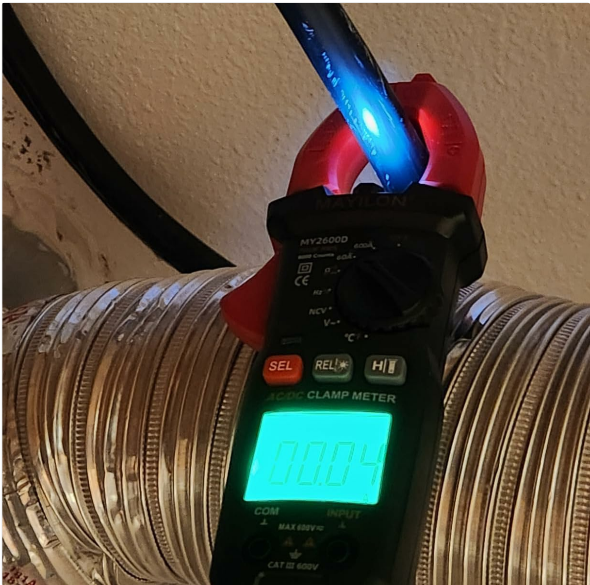
Image 6.1: The clamp meter in use, measuring current on a single conductor.
