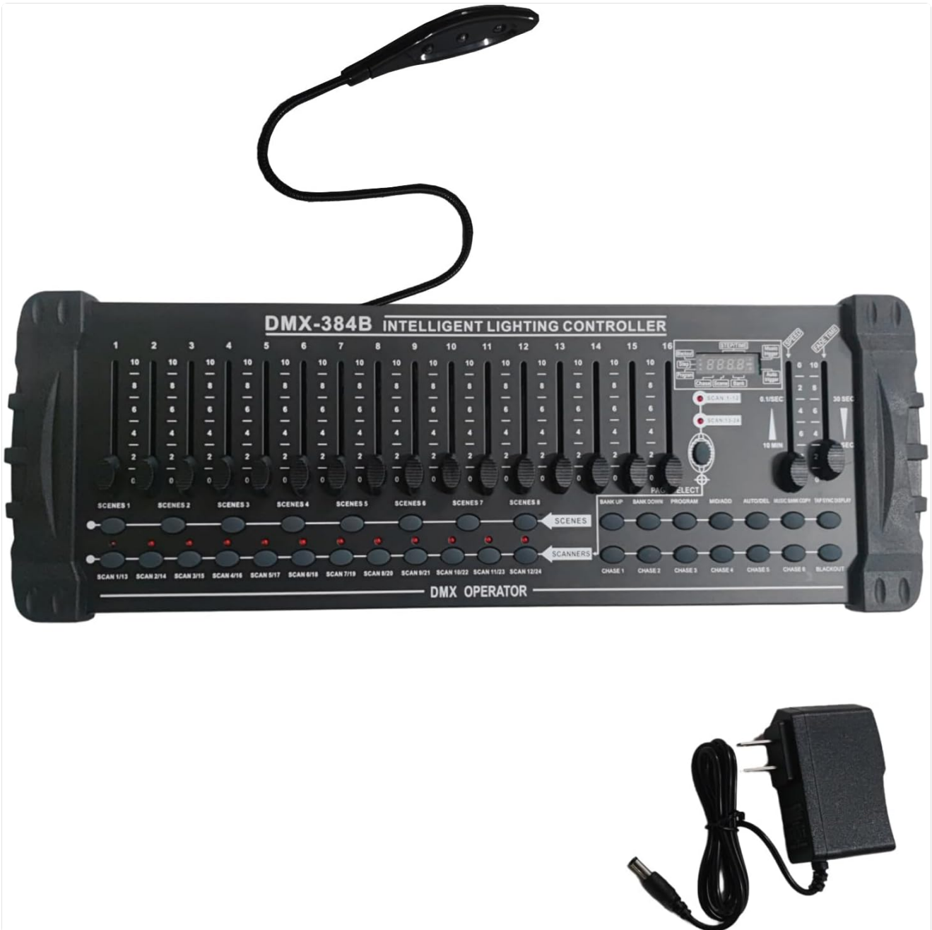
Figure 2.2.1: Contents of the package including the DMX controller, power adapter, and gooseneck LED light.
