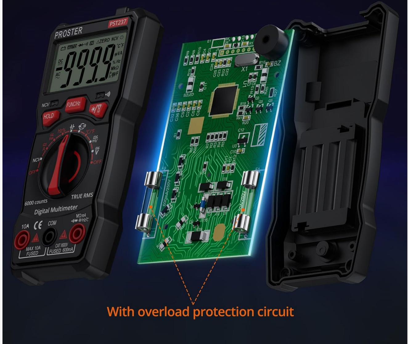
Image: Internal view of the multimeter highlighting its smart protection features, including built-in double safety tubes and an overload protection circuit.
