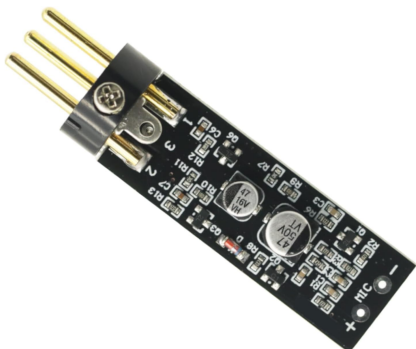
Figure 2: Angled perspective of the amplifier board, illustrating the three gold-plated output pins for connection to an XLR input.
