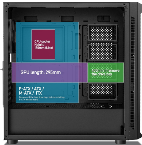
Image: Internal clearances for CPU cooler (max 180mm height), GPU (295mm, 400mm if drive bay removed), and motherboard sizes (E-ATX, ATX, M-ATX, ITX).
