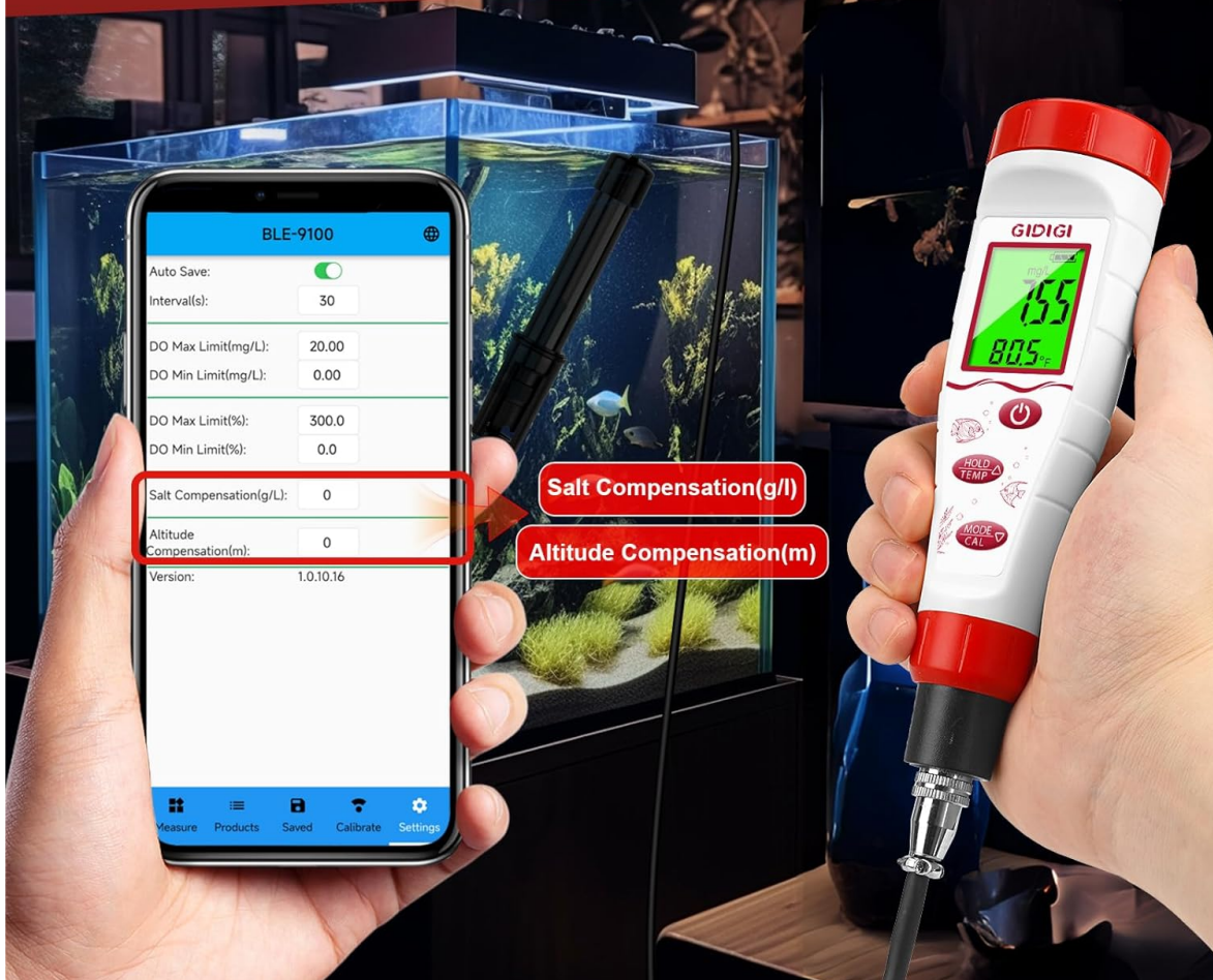
Image: Bluetooth Dissolved Oxygen Tester with App. This image illustrates the meter connected via Bluetooth to a smartphone app, showing options for salinity and altitude compensation settings.
