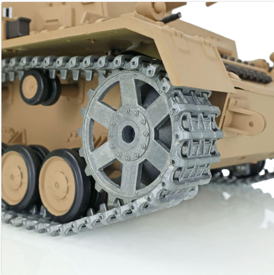
Detailed view of the metal tracks and drive sprocket, emphasizing the robust construction.
