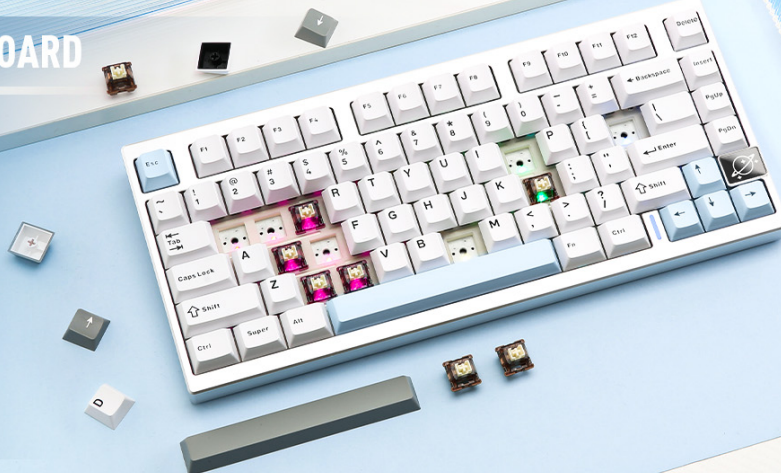
Image: Detailed view of the hot-swappable feature, showing switch types and south-facing LEDs.
