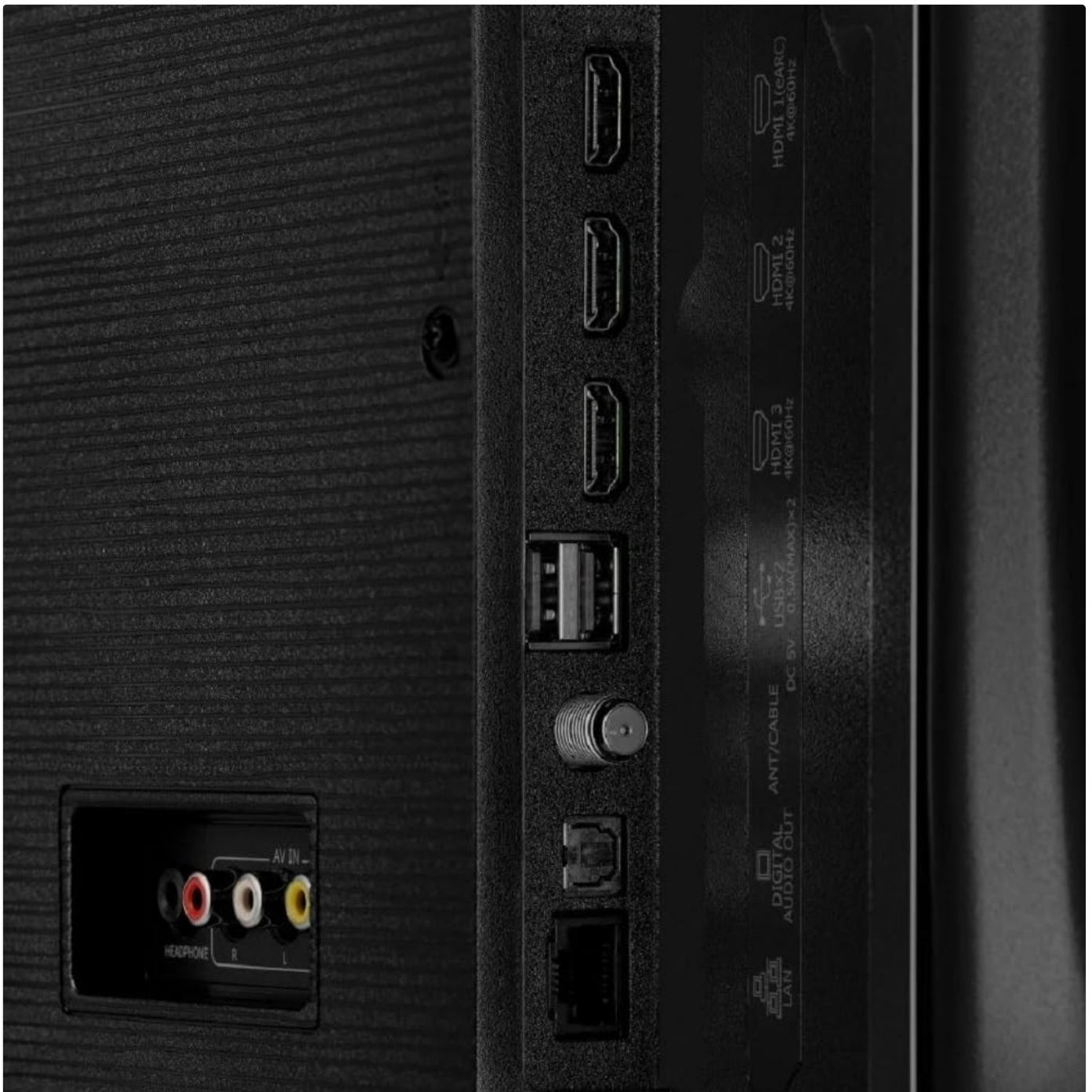
Image: Rear view of the Hisense TV, highlighting the HDMI, USB, Antenna/Cable, Digital Audio Out, and Ethernet ports.
