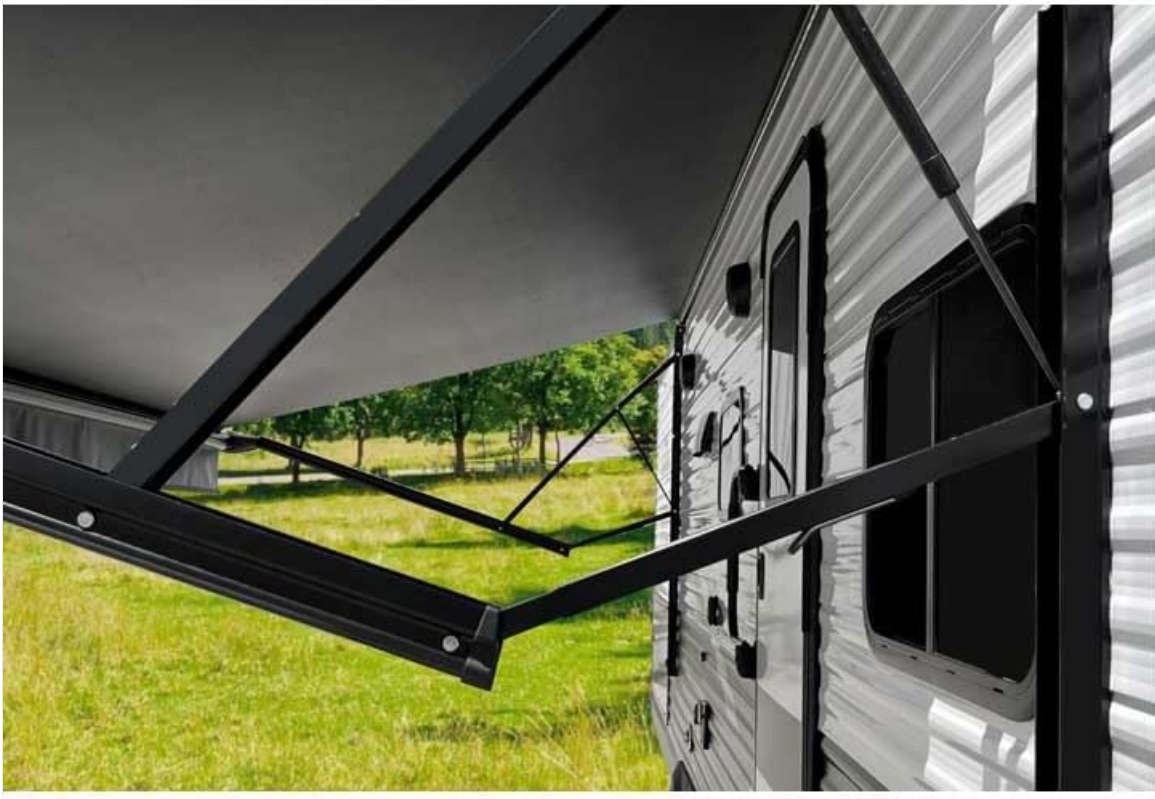
Figure 1: Velarium 68" Power/Idler Arm installed on an RV with awning extended. This image shows the robust extruded arms supporting the awning fabric.
