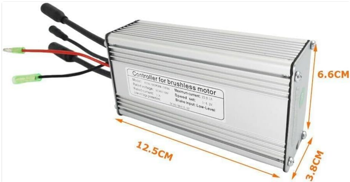
Image 3.1: Controller dimensions (approximately 12.5cm x 6.6cm x 3.8cm) for installation planning.
