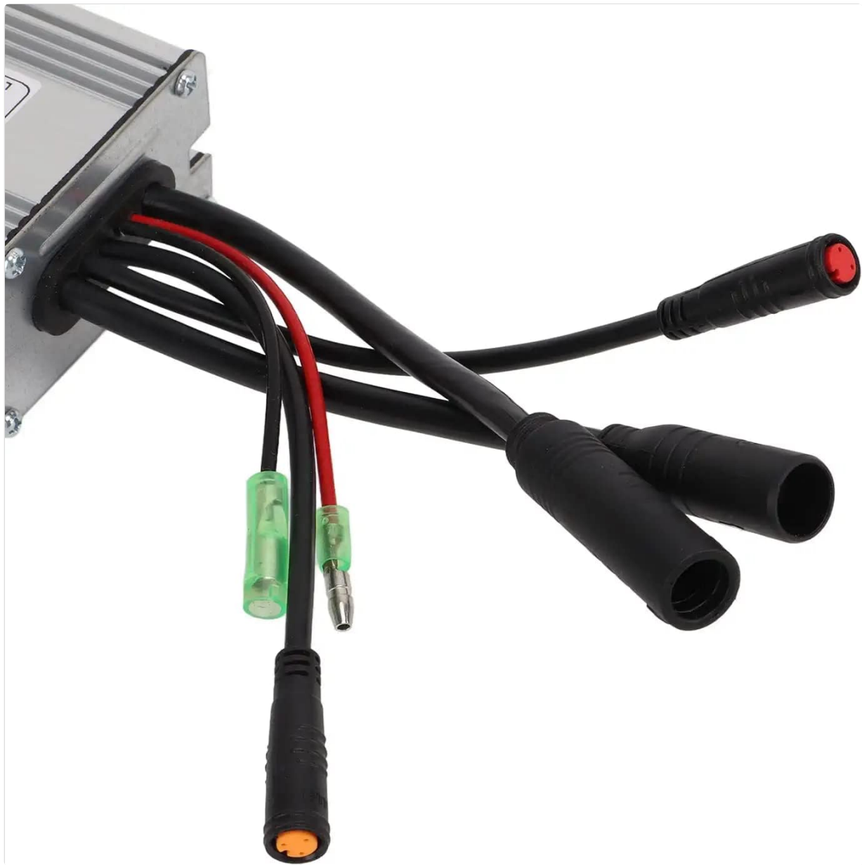
Image 3.3: Close-up view of the controller's connectors, showing the various wire types and their corresponding functions.
