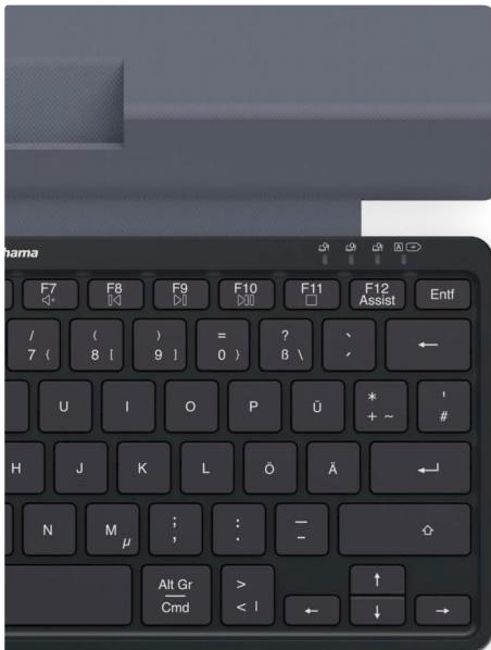
Close-up of the right side of the Hama Travel 600 keyboard, detailing the function keys (F7-F12), multimedia controls, and the QWERTZ key arrangement, including the 'Alt Gr' and 'Cmd' keys.
