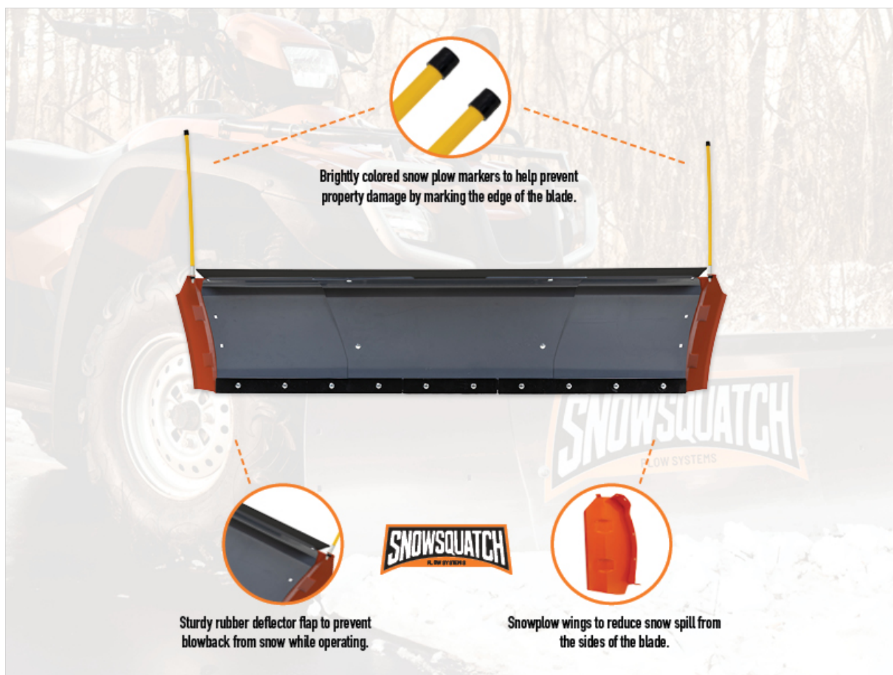
Figure 4.4: Plow system attached to a UTV, ready for winch connection.
