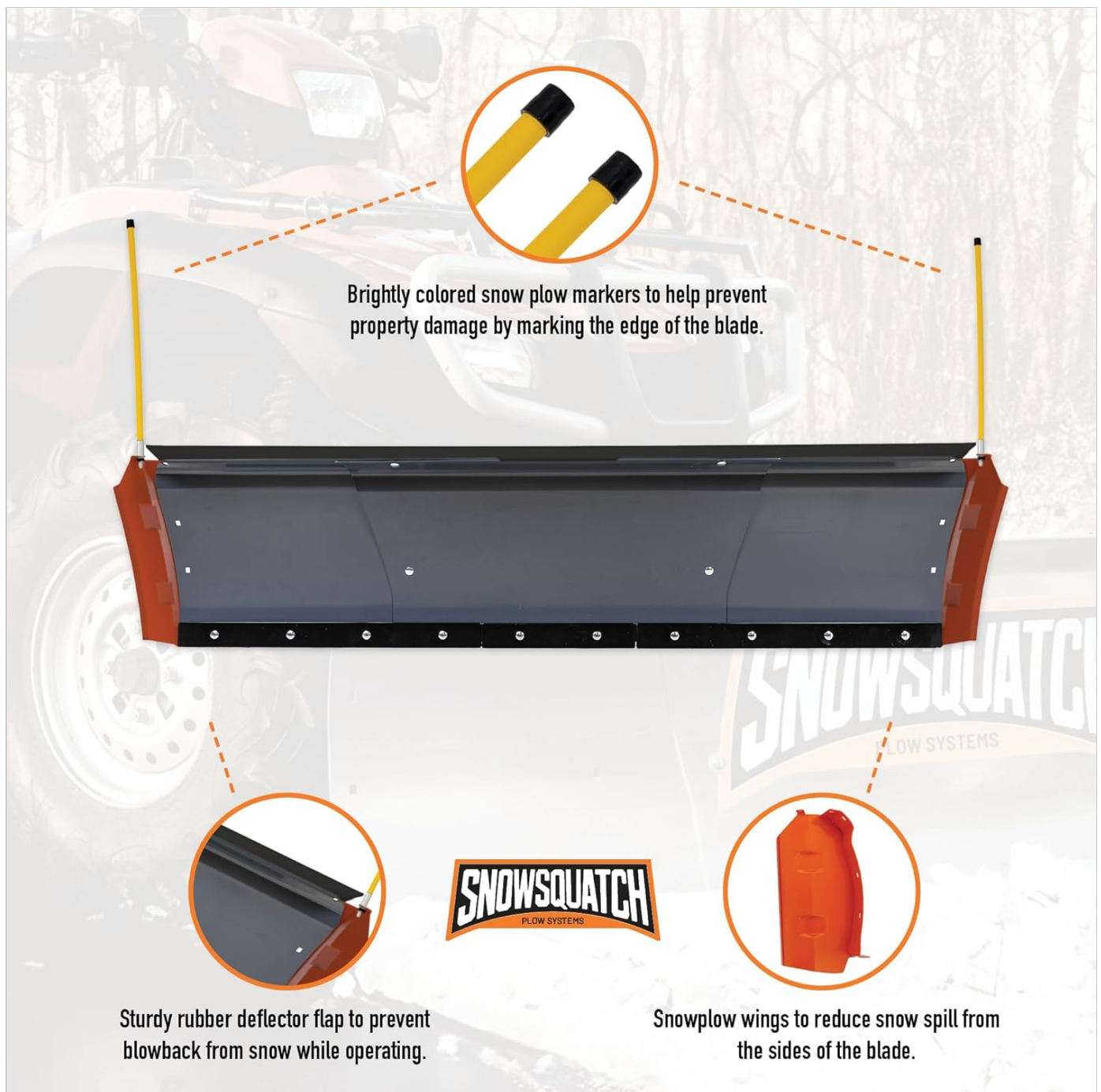
Figure 5.4: Plow markers, rubber deflector, and side wings.
