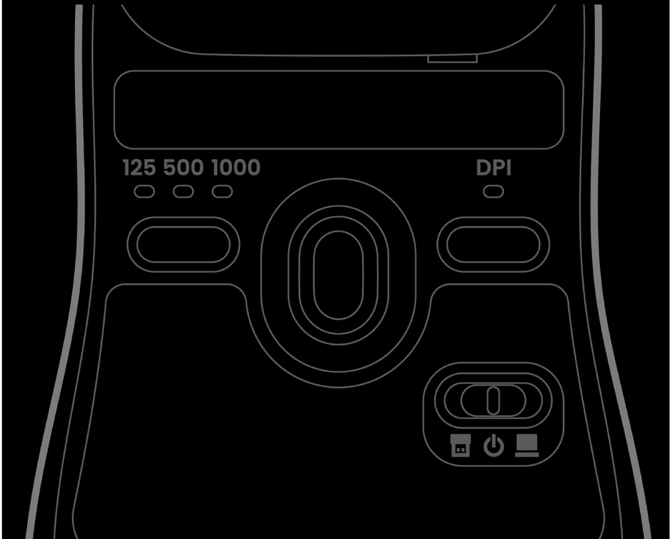
Figure 6.1: Bottom panel controls for DPI and Polling Rate adjustments.
