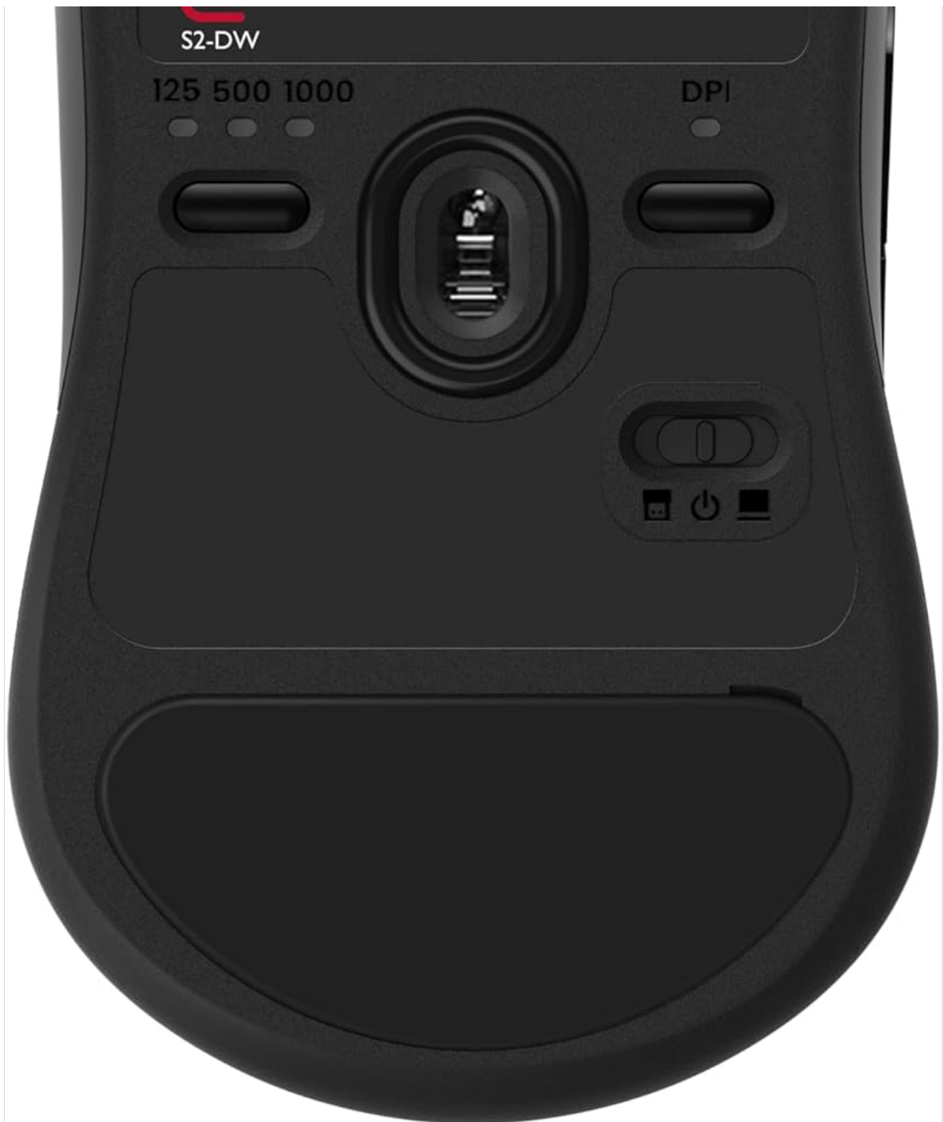
Figure 4.3: Bottom view displaying the DPI and Polling Rate switches, and the optical sensor.
