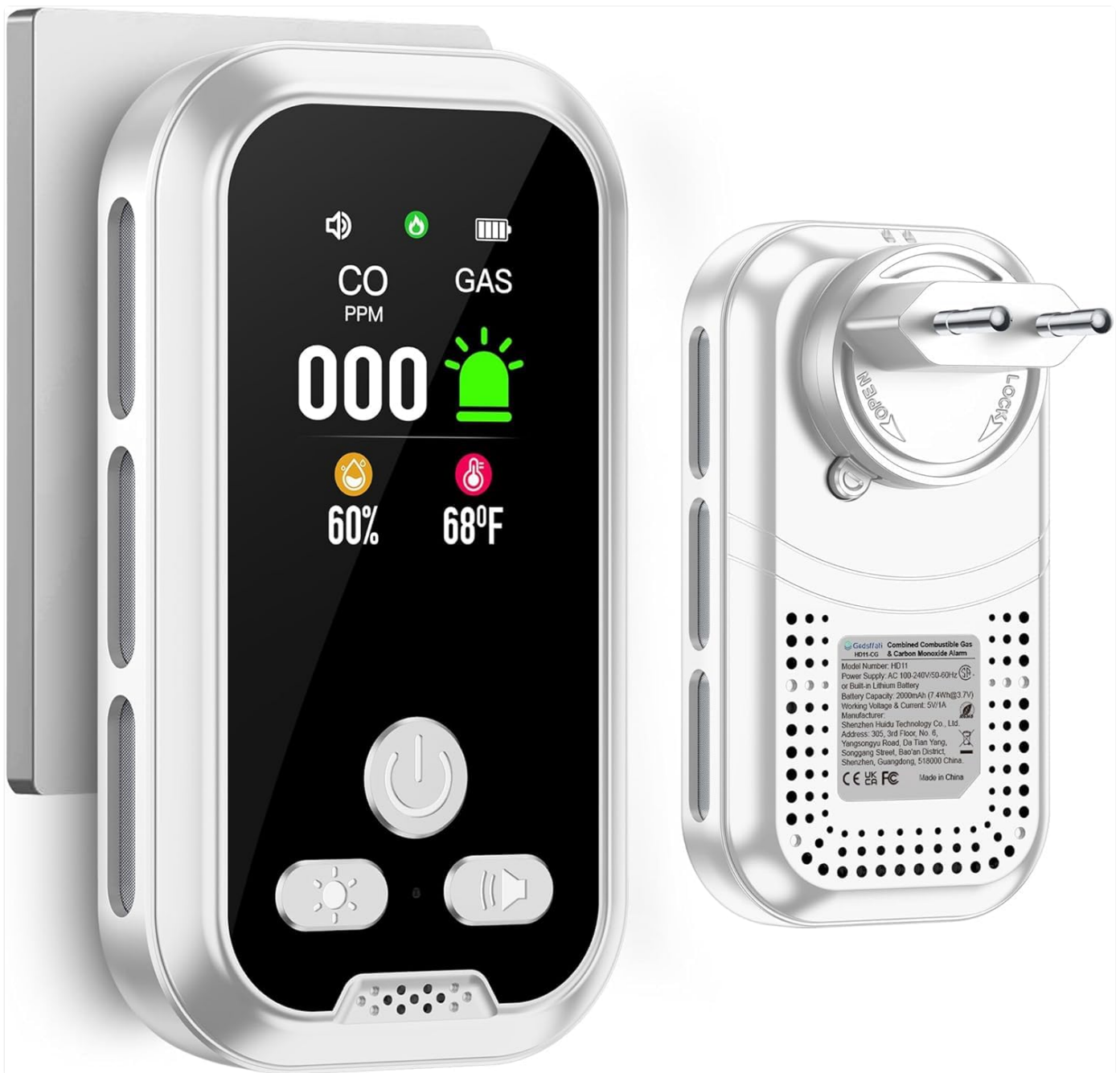
Image: Gedsffati HD11-CG Gas and CO Detector, front and back view with plug adapter.
