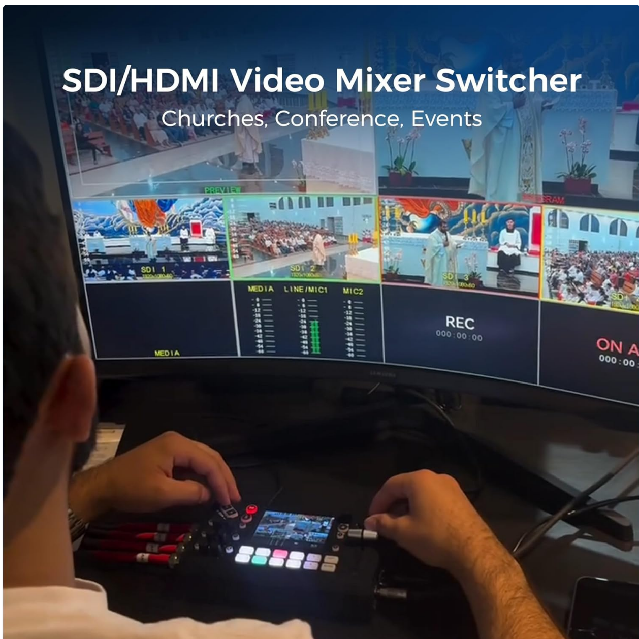
Figure 3: The 3.5-inch touchscreen displaying a multiview of inputs.
