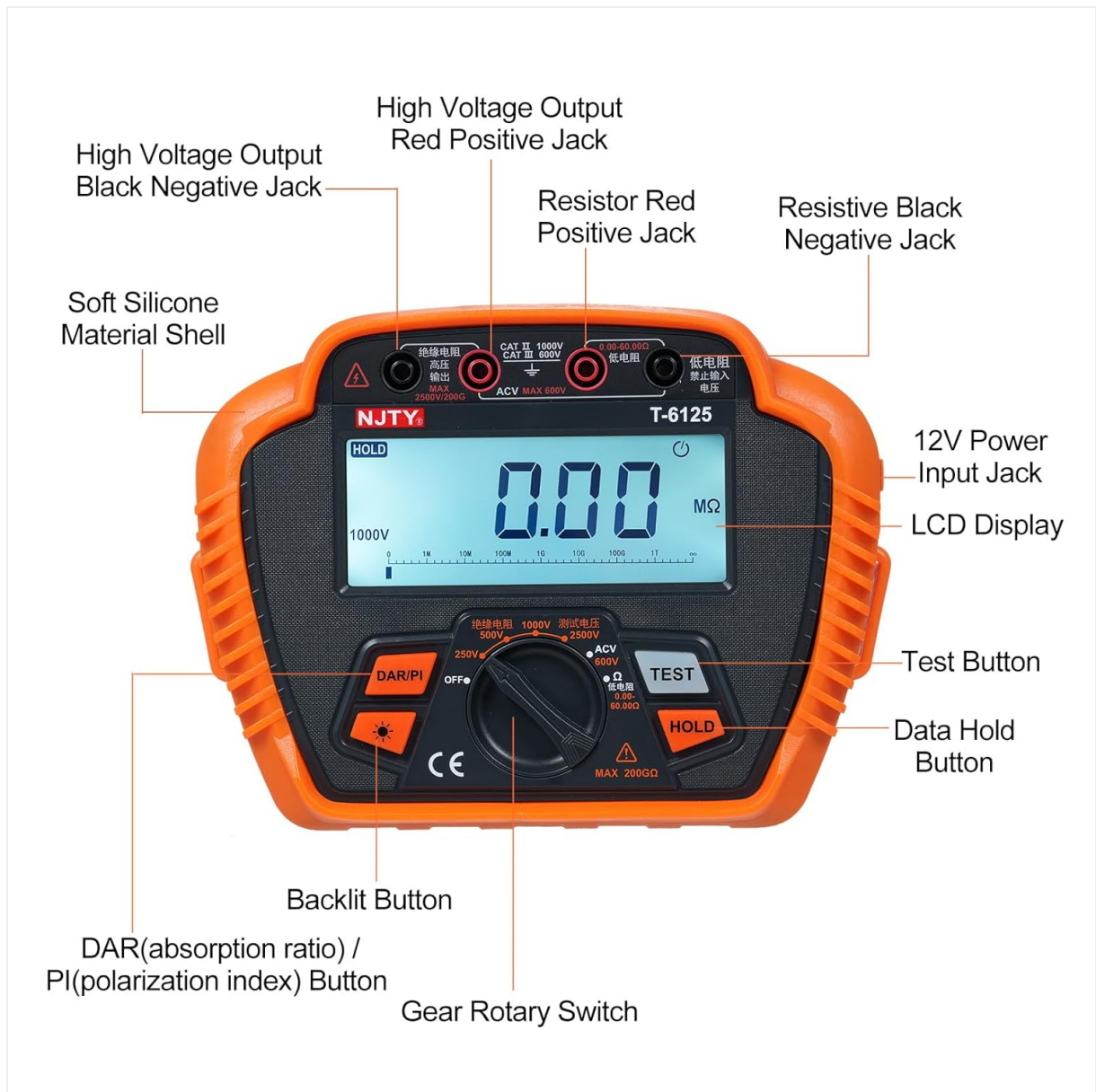
Figure 2: Front panel layout and key components of the T6125.
