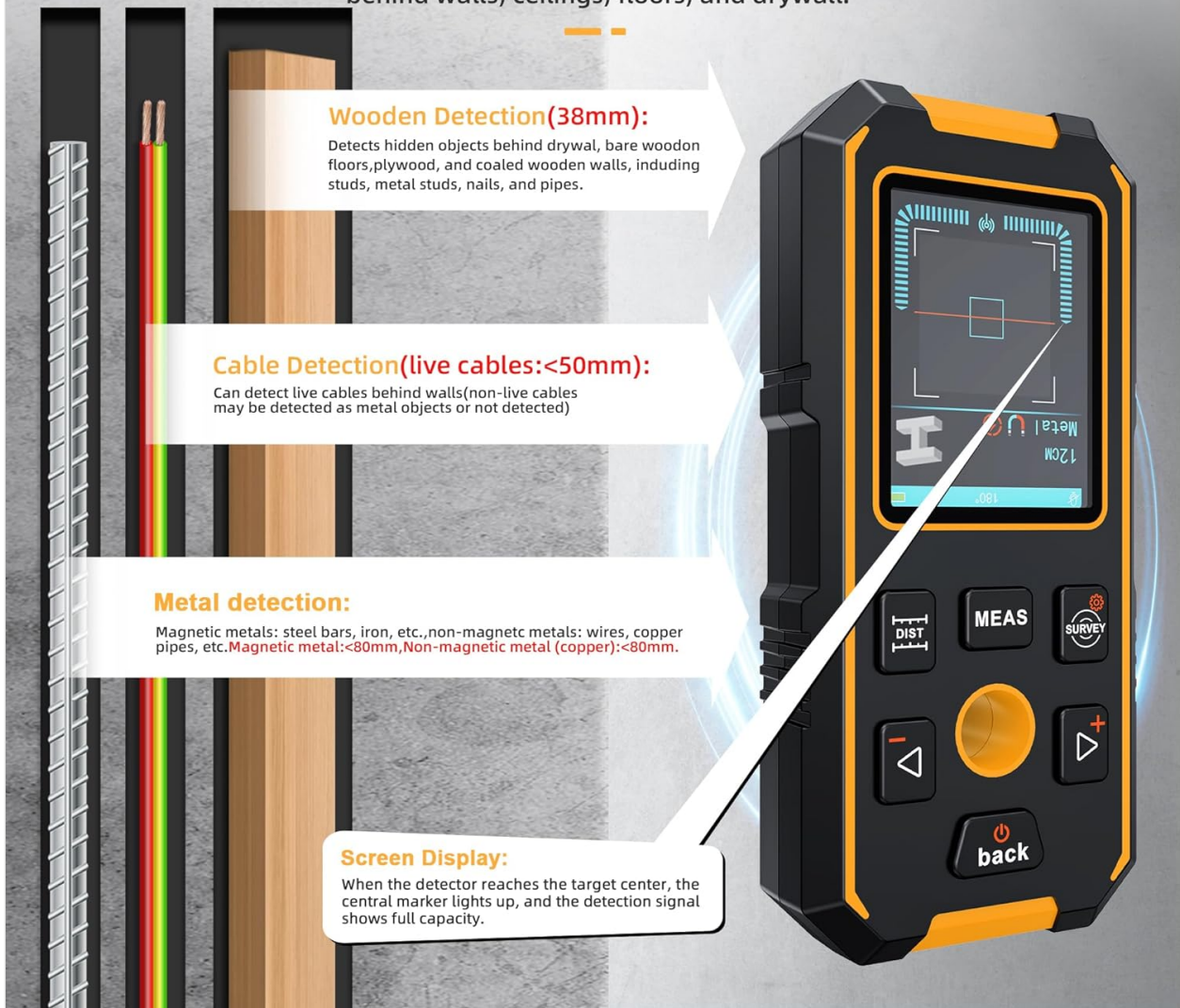
Figure 3: Overview of Wood, Cable, and Metal Detection Capabilities
