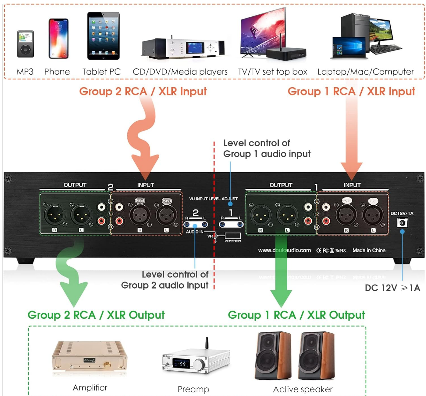
Image: Diagram of the Douk Audio VU4 rear panel, showing input and output connections for RCA and XLR for both Group 1 and Group 2, along with the DC 12V power input and VU Input Level Adjust.
